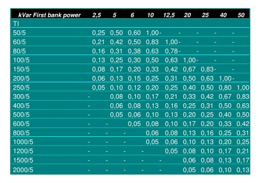
When using the regulator on 220/240 Vac networks the C/K values should be doubled. " - " means primary current of the TI is too small.
